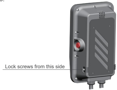
Charger box locking on back plate diagram
